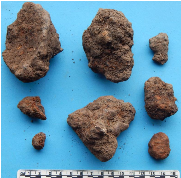
PL. 1.15. Furnace bottom (top left) and iron slag. Context 106.
